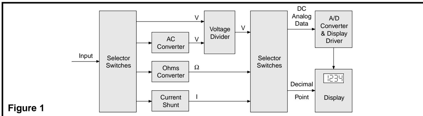
For resistance measurements, an internal voltage source drives the test resistor in series with a known resistor. The ratio of the test resistor voltage to the known resistor voltage is used to determine the value of the test resistor.
