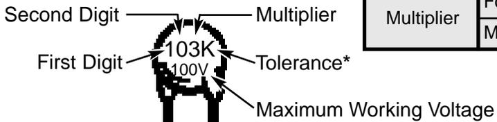
The value is  $10 \times 1,000 = 10,000\text{pF}$  or  $.01\mu\text{F}$  100V
