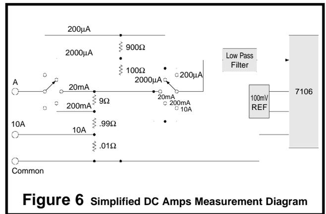
**Figure 6** Simplified DC Amps Measurement Diagram
