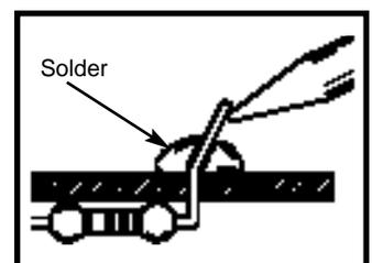
4. **Solder bridges** - occur when solder runs between circuit paths and creates a short circuit. This is usually caused by using too much solder. To correct this, simply drag your soldering iron across the solder bridge as shown.
